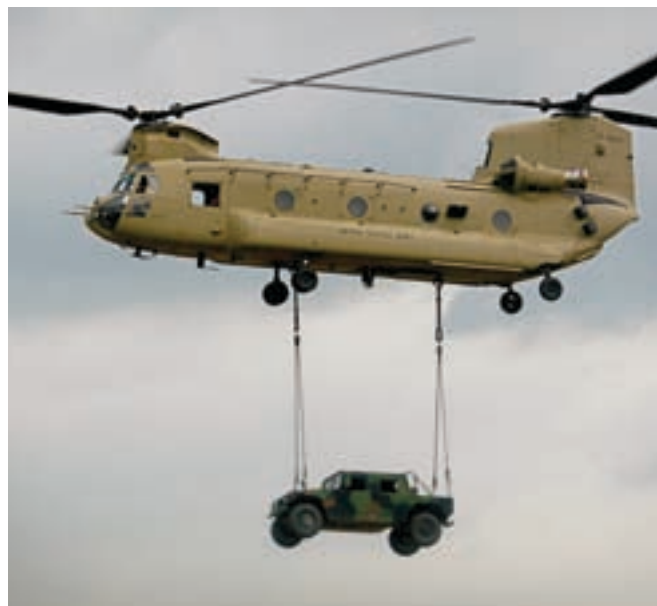
CH-47F CONDUCTING AN OT MISSION AT FT. CAMPBELL, KY IN MARCH 2007. OT CONSISTED OF 18 MISSIONS AND OVER 60 HOURS TESTING, SIMULATING A WIDE RANGE OF AIR ASSAULT, COMBAT RESUPPLY AND TRANSPORT MISSION SCENARIOS IN A GWOT MISSION ENVIRONMENT.
