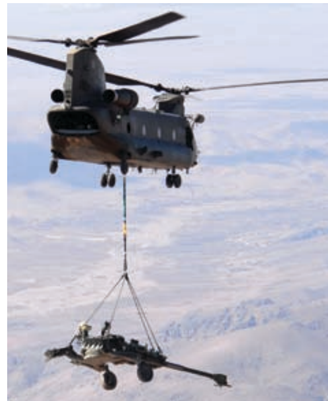
RAF 1310FLT CHINOOKS SEEN OPERATING IN SUPPORT OF THE ROYAL CANADIAN HORSE ARTILLERY (RCHA) DURING AN ISAF MISSION IN THE MOUNTAINS NORTH OF KANDAHAR. CHINOOKS MOVED THEIR M777, 155MM HOWITZERS, AMMUNITION AND SUPPLIES IN SUPPORT OF AN ISAF LED MISSION.
